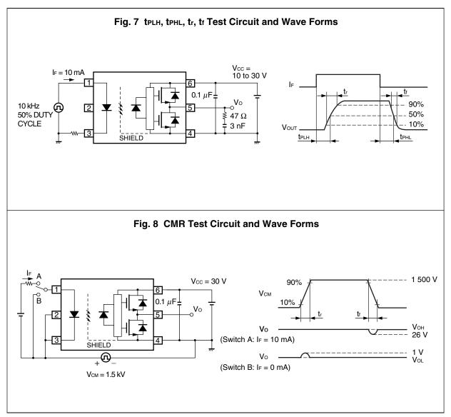
**Remarks 1.** Common Mode Transient Immunity at High Level Output is the maximum value of  $dV_{CM}/dt$  at which the output remains High Level (e.g.  $V_O > 15 \text{ V}$ ).
