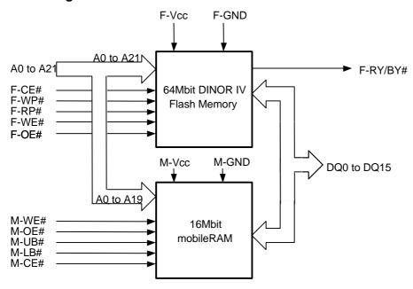
Note: In the data sheet there are "VCC"s , "GND"s , "OE"s and "WE"s. In the Flash Memory part they mean F-Vcc, F-GND, F-OE and F-WE. In the mobileRAM part they mean M-Vcc, M-GND, M-OE and M-WE.
