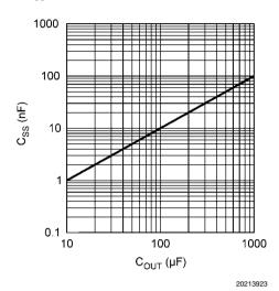
FIGURE 2. Typical C<sub>SS</sub> vs C<sub>OUT</sub> Values
