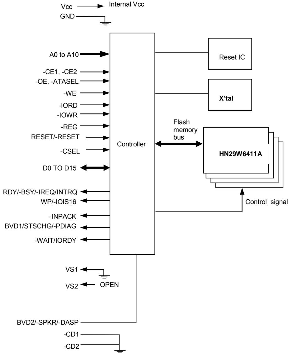
Note: -CE1, -CE2, -OE, -WE, -IORD, -IOWR, -REG, RESET, -CSEL pins are pulled up in the card.
