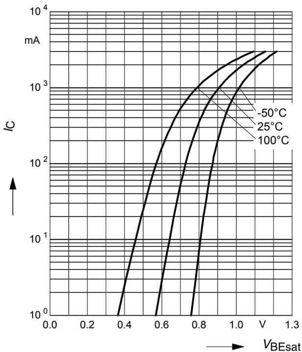
**Collector current  $I_C = f(V_{BE})$**
