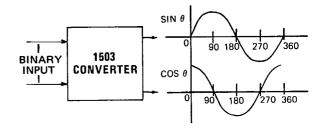
This solid state model converts a 14 bit digital input into two AC output voltages that are proportional to the sine and cosine of the indicated input angle, and is therefore ideally suited for radar display systems, computing applications, or to drive power amplifiers for D/S application. Separate logic and analog grounds can be supplied to minimize potential ground loop problems.
