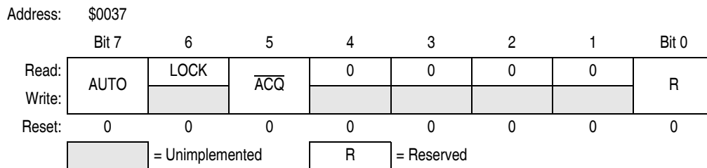
Figure 4-5. PLL Bandwidth Control Register (PBWC)
