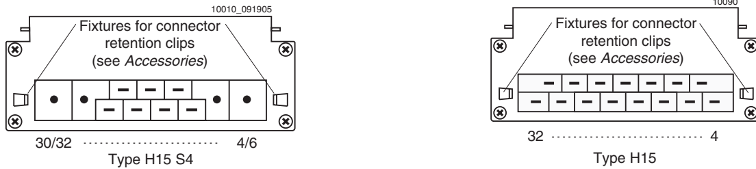
Fig. 21 View of converter's male connectors
