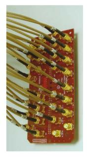
adaptors provide a convenient conversion from SMA to the evaluation board's 0.1" headers. This alleviates the simultaneous removal of 28 SMAs (14-bit differential LVDS) when required to be disconnected. One advantage of this is the ability to easily swap the data generator between DAC data ports if insufficient channels are available to drive both ports simultaneously.
