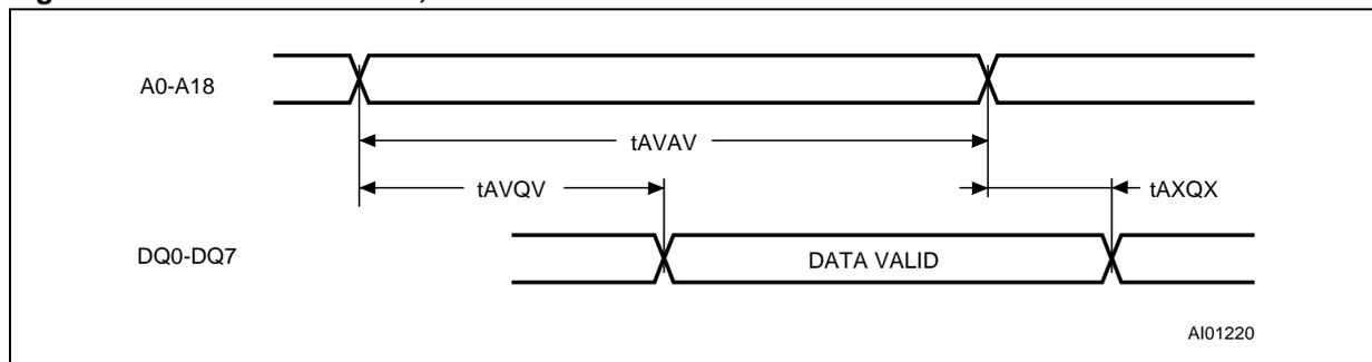
Note: Chip Enable ( $\overline{E}$ ) and Output Enable ( $\overline{G}$ ) = Low, WRITE Enable ( $\overline{W}$ ) = High.
