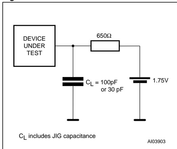
Note: Excluding open drain output pins; 50pF for M48Z512AV.
