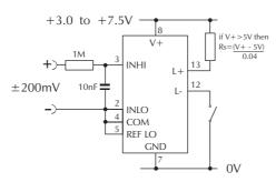
Measuring an input voltage referenced to a floating supply, i.e. the input voltage and the meter's power supply are isolated from each other.
