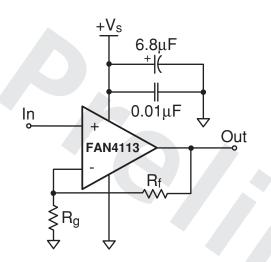
Figure 1: Typical Non-inverting Configuration
