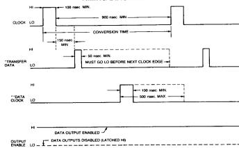
"IF TRANSFER DATA IS HELD HI, THEN THE COUNTER OUTPUTS APPEAR DIRECTLY AT THE BIT OUTPUTS "DRIVEN FOR SERIAL DATA OUTPUT ONLY.
