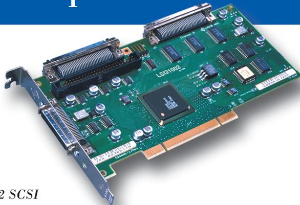
*The LSI21002 PCI-to-Ultra2 SCSI dual channel host adapter supports a wide variety of Fast and Ultra SCSI devices.*
