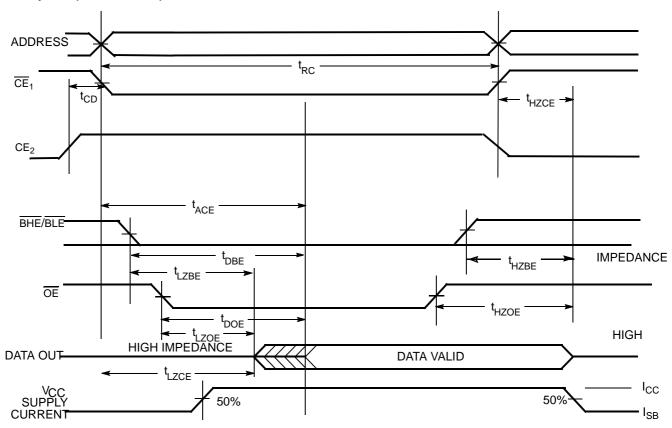
Notes: 16. Whenever  $\overline{CE}_1$  = HIGH or  $CE_2$  = LOW, BHE/BLE are taken inactive, they must remain inactive for a minimum of 5 ns. 17. Device is continuously selected.  $\overline{OE} = \overline{CE}_1 = V_{|L}$  and  $CE_2 = V_{|H}$ .
