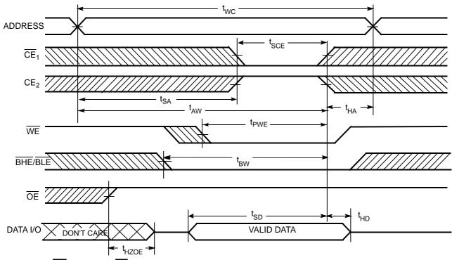
Write Cycle 3 ( $\overline{\text{WE}}$  Controlled,  $\overline{\text{OE}}$  LOW)<sup>[16, 21]</sup>
