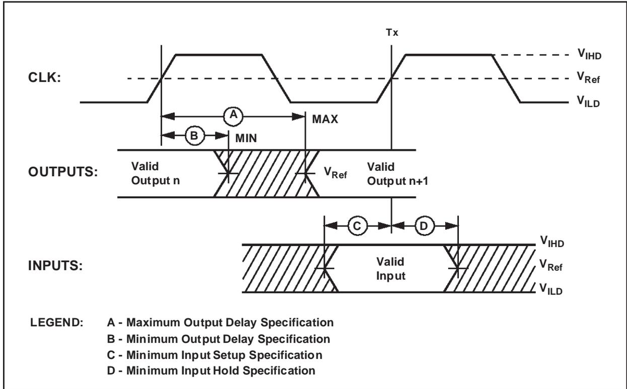
**Figure 9. CLK Timing Measurement Points**
