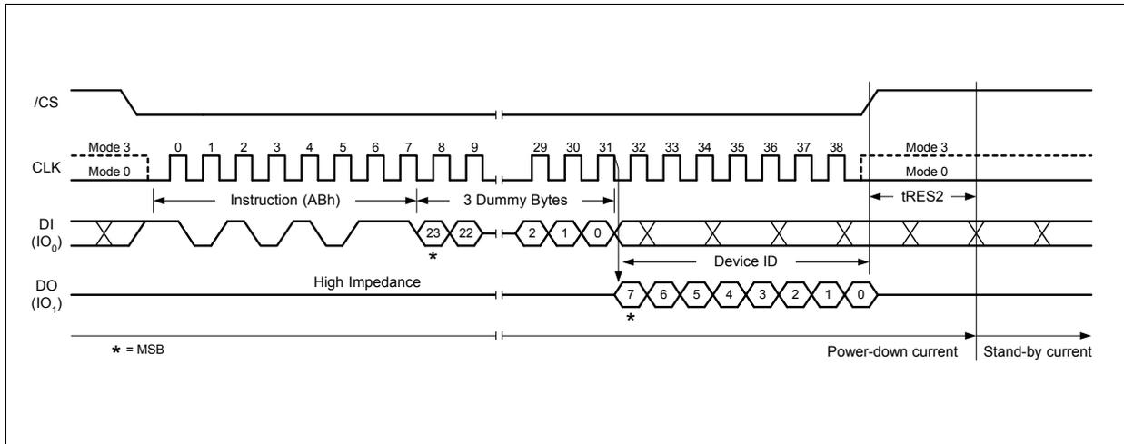
Figure 21. Release Power-down / Device ID Instruction Sequence Diagram
