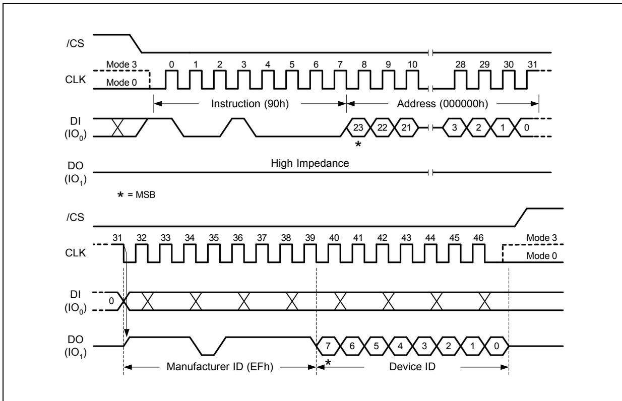
Figure 22. Read Manufacturer / Device ID Diagram
