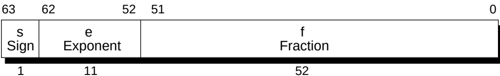
Figure 7-6 Double-Precision Floating-Point Format
