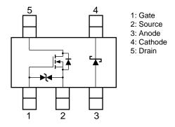
**Remark** The diode connected between the gate and source of the transistor serves as a protector against ESD.
