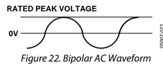
Figure 22. Bipolar AC Waveform
