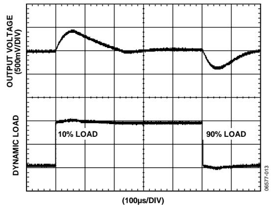
Figure 10. Typical Transient Load Response, 3 V Output, 10% to 90% Load Step
