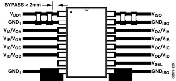
Figure 17. Recommended Printed Circuit Board Layout
