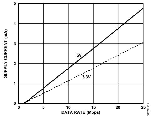
Figure 15. Typical  $I_{ISO(D)}$  Dynamic Supply Current per Input
