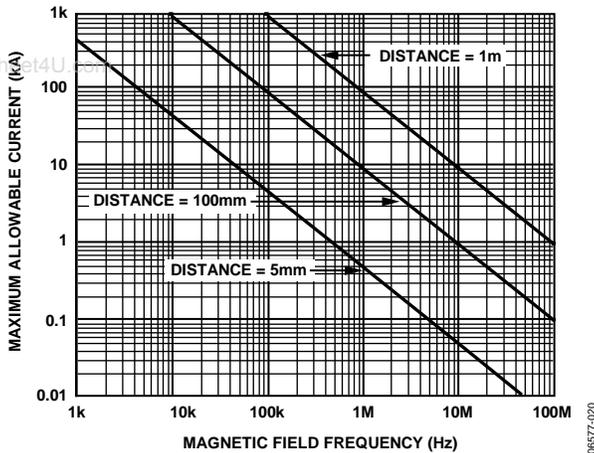
Figure 20. Maximum Allowable Current for Various Current-to-ADuM5400 Spacings
