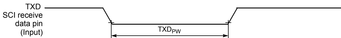
Figure 10-18 TXD Pulse Width
