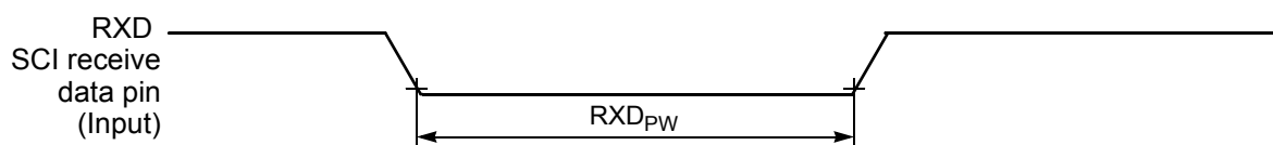
Figure 10-17 RXD Pulse Width
