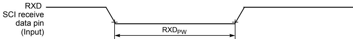
Figure 10-16 RXD Pulse Width
