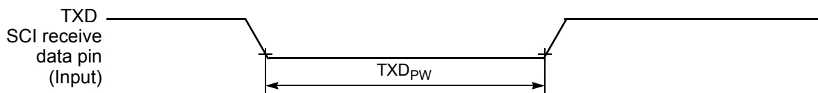
Figure 10-17 TXD Pulse Width
