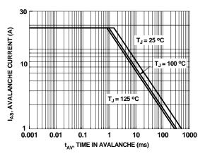
Figure 9. Unclamped Inductive Switching Capability
