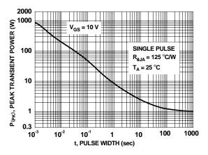
Figure 12. Single Pulse Maximum Power Dissipation
