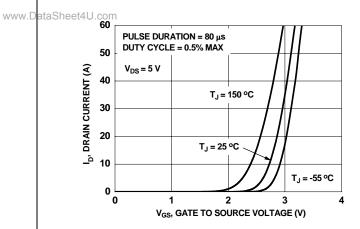
Figure 5. Transfer Characteristics
