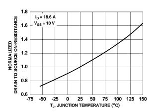
Figure 3. Normalized On-Resistance vs Junction Temperature
