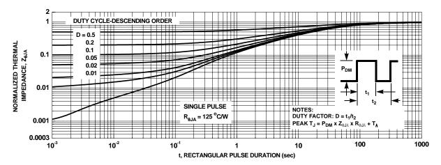
Figure 13. Transient Thermal Response Curve
