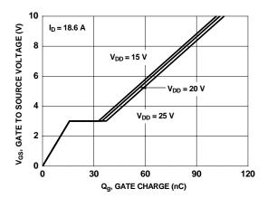
Figure 7. Gate Charge Characteristics
