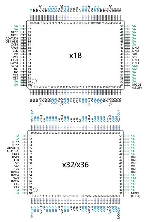
\*No Connect (NC) is used on the x32 version. Parity (DQPx) is used on the x36 version. \*\*Pins 83 and 84 are reserved for address expansion, 8Mb and 16Mb respectively.
