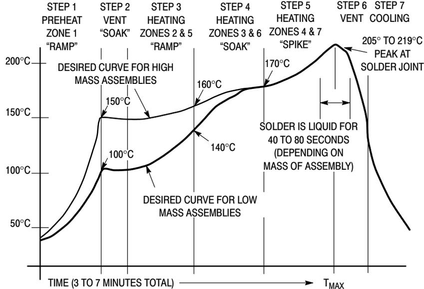
**Figure 8. Typical Solder Heating Profile**
