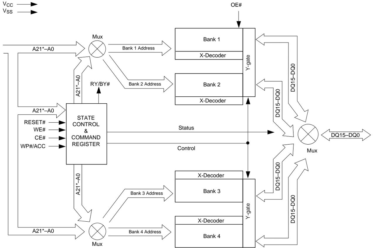
\* Addresses for Am29DL640G are A21-A0. Address for Am29DL320G are A20-A0.
