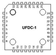
NOTE: Bottom Pad for MLF Package Should be Soldered to Ground.
