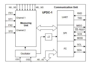
The UFDC-1 can be easy included into digital environment, controlled by an external microcontroller (slave mode) or work independently as a separate measuring unit without an external control (master mode). The function selection can be configured in both software and hardware.
