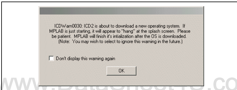
FIGURE 3-2: UPDATING MPLAB ® ICD 2 FIRMWARE DIALOG
