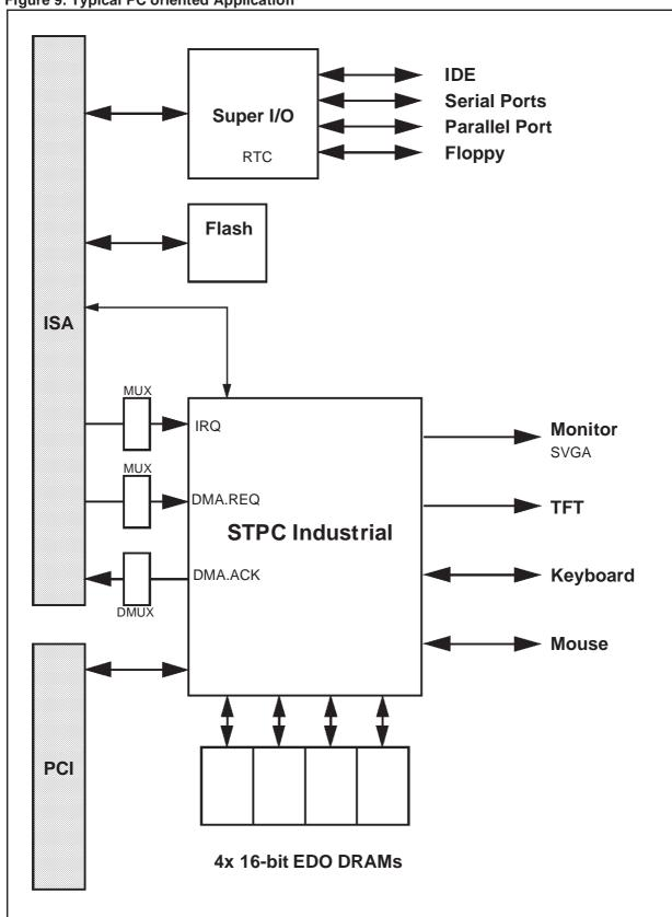
Figure 9. Typical PC oriented Application
