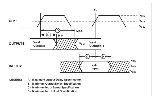
Figure 13. CLK Timing Measurement Points
