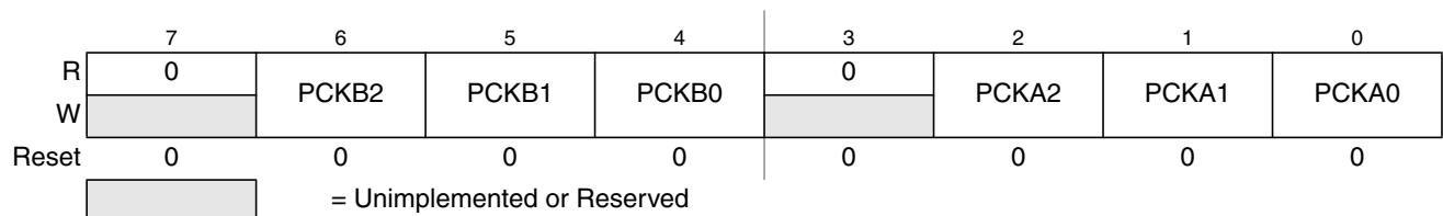
Figure 17-6. PWM Prescale Clock Select Register (PWMPRCLK)
