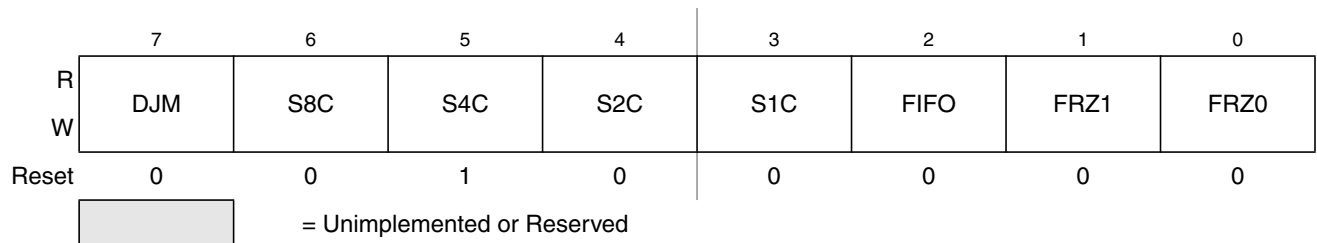
Figure 14-6. ATD Control Register 3 (ATDCTL3)
