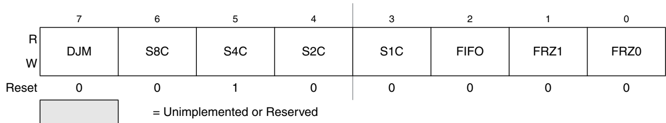
Figure 12-6. ATD Control Register 3 (ATDCTL3)
