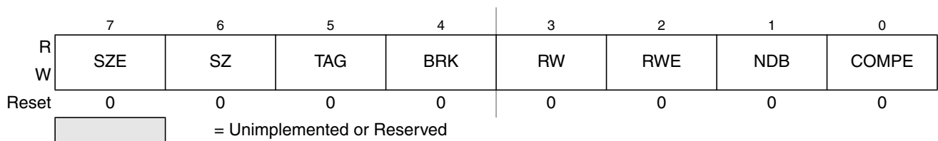
Figure 8-13. Debug Comparator Control Register DBGACTL (Comparator A)
