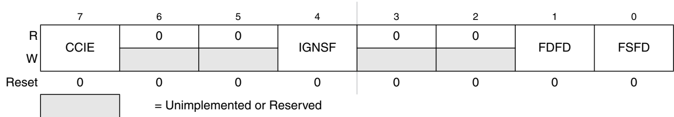
Figure 23-9. Flash Configuration Register (FCNFG)
