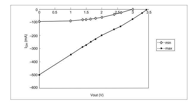
DC Characteristics (Ta = 0 to 55°C,  $V_{CC}$  = 3.3 V  $\pm$  0.3 V,  $V_{SS}$  = 0 V)
