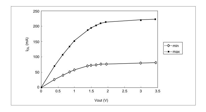
Output High Current  $(I_{OH})~(Ta=0~to~55^{\circ}C,~V_{CC}=3.0~V~to~3.45~V,~V_{SS}=0~V)$
