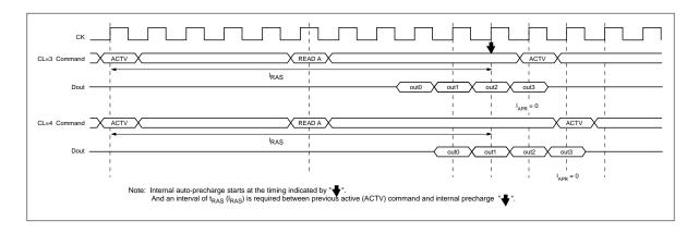
**Write with auto-precharge:** In this operation, since precharge is automatically performed after completing a burst write or single write operation, a precharge command need not be executed after each write operation. The command executed for the same bank after the execution of this command must be the bank active (ACTV) command. In addition, an interval of  $l_{APW}$  is required between the final valid data input and input of next command.
