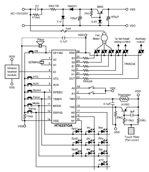
Note:  $C1=2\mu F/300V$  when the AC power supply is 110V.
