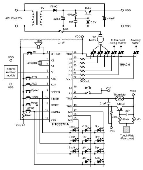
Note: Typical infrared receiver modules: PIC-12043T/PIC-12043S (KODENSHI CORP.) or LTM9052 (LITEON CORP.)
