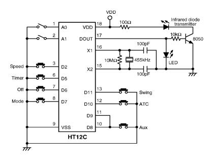
\* Note: Typical infrared diode—EL-1L2 (KODENSHI CORP.)
