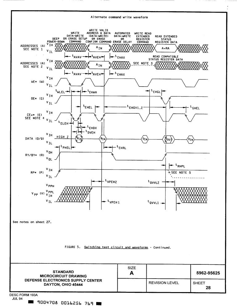
WE# and CE# controlled page buffer write timing waveforms respectively
