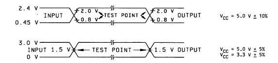
NOTES: AC testing ( $V_{CC}$  = 5.0 V  $\pm$  10%): Inputs are driven at  $V_{OH}$  (2.4 VTTL) for a logic "0". Input timing begins at  $V_{IH}$  (2.0 VTTL) and  $V_{IL}$  (0.8 VTTL). Output timing ends at VIH and VIL. Input rise and fall times (10% to 90%) < 10 ns.
