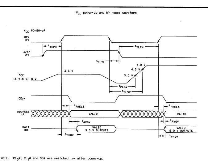
FIGURE 5. Switching test circuit and waveforms - continued.
