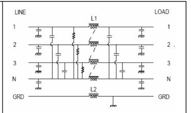
Operating Voltage = 250/480 V~, 50 / 60 Hz Operating Voltage = 125/208 V~, 50 – 400 Hz Operating Current = 100 A / Phase Temperature Range = -20 TO 50 Deg. C Diel. Withstand (L-CASE) = 1500 V~ FOR 1 MIN. Diel. Withstand (L-L) = 1500 Vdc For 1 Min. Leakage Current = 2.2 ma @ 250 V~, 60 Hz
