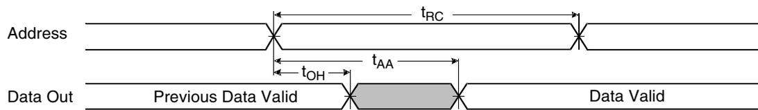
Note: CE1#s = OE# =  $V_{IL}$ , CE2s = WE# =  $V_{IH}$ , UB#s and/or LB#s =  $V_{IL}$
