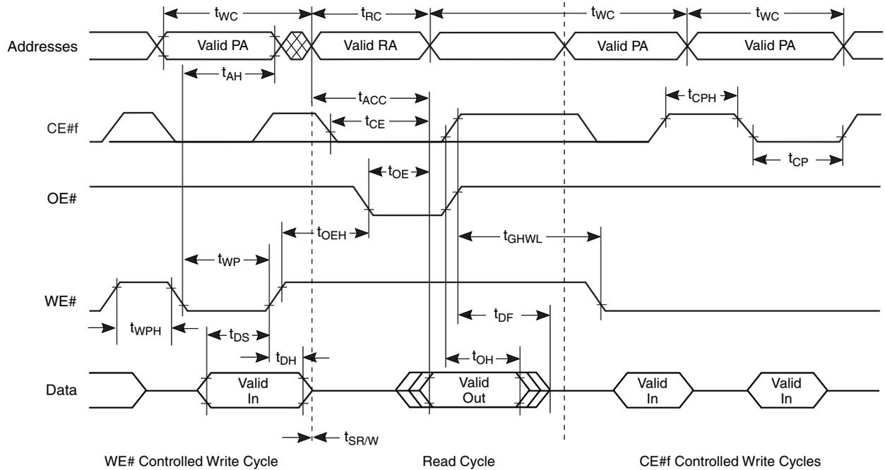
Figure 22. Back-to-back Read/Write Cycle Timings
