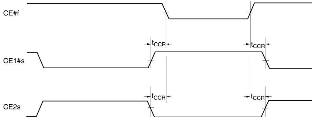
Figure 14. Timing Diagram for Alternating Between SRAM to Flash
