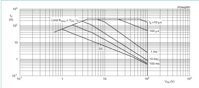
$T_{mb} = 25^{\circ}C$ ;  $I_{DM}$  is a single pulse
