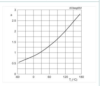
$a = \frac{R_{DSon}}{R_{DSon(25^{\circ}C)}}$
