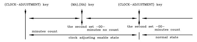
2. In case the (MEMORY(CLOCK-ADJUSTMENT)) key is pushed again within 1 minute from the setting the clock adjusting enable state.
