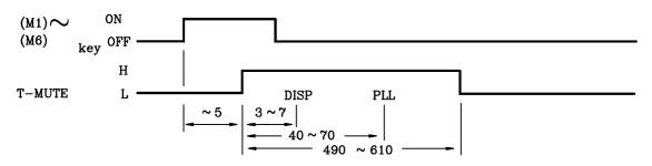
In case of calling the preset memory directly (In case that band changed)
