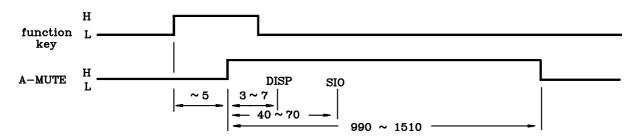
\* function key: (TAPE)key. (TUNER)key. (AUX)key. (PHONO)key. (CD)KEY. (VCR)key. (TV)key
