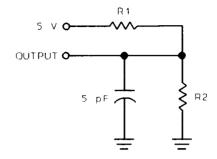
Circuit A Output load Circuit B Output load for  $\mathbf{t}_{\mbox{HZCS}}$
