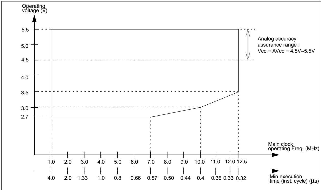
**Figure 3 Operating Voltage vs. Main Clock Operating Frequency (MB89PV480)**
