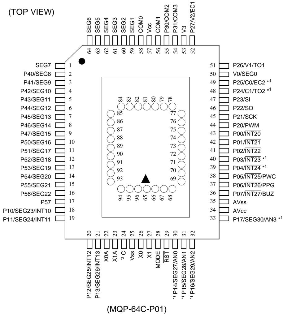
\*1: If booster is selected, EC2 and TO2 will be redirected to P03/ $\overline{\text{INT23}}$  and P04/ $\overline{\text{INT24}}$  respectively.
