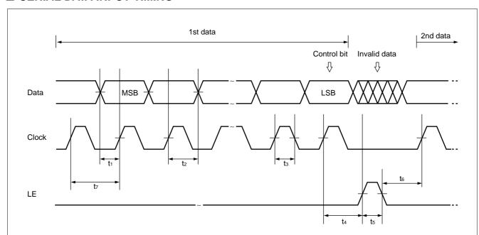
On the rising edge of the clock, one bit of data is transferred into the shift register.
