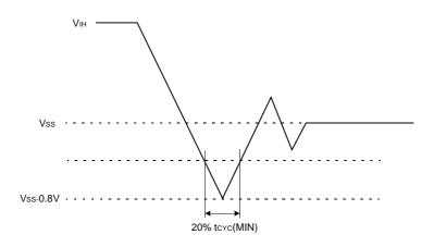
**TEST CONDITIONS** (TA=0 to 70°C, VDD=2.5V  $\pm$ 5%, unless otherwise specified)
