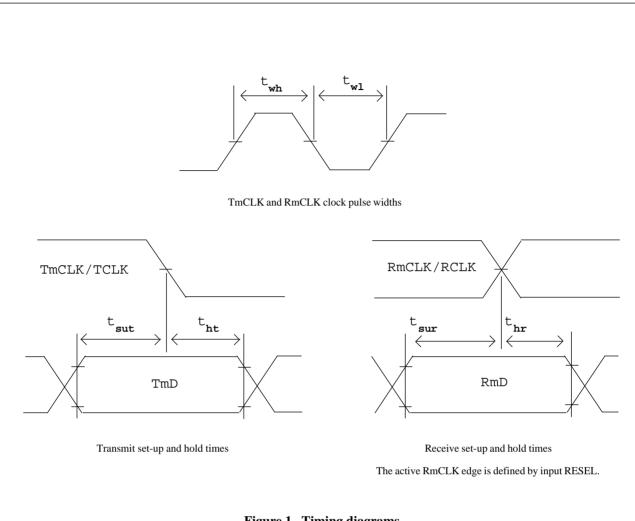
Figure 1. Timing diagrams
