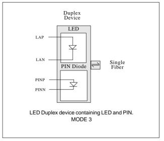
LASER = GND LASRX = GND PINRX = VA+
