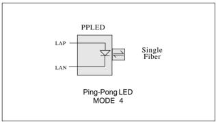
LASER = GND LASRX = VA+ PINRX = GND
