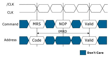
Code = Mode Register / Extended Mode Register selection (BA0, BA1) and op-code (A0 - An)
