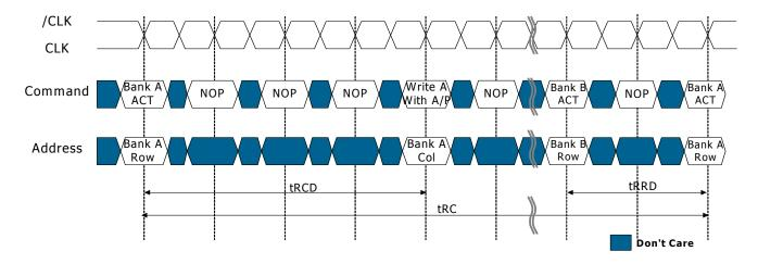
Once a row is Open(with an ACTIVE command) a READ or WRITE command may be issued to that row, subject to the tRCD specification. tRCD (MIN) should be divided by the clock period and rounded up to the next whole number to determine the earliest clock edge after the ACTIVE command on which a READ or WRITE command can be entered.
