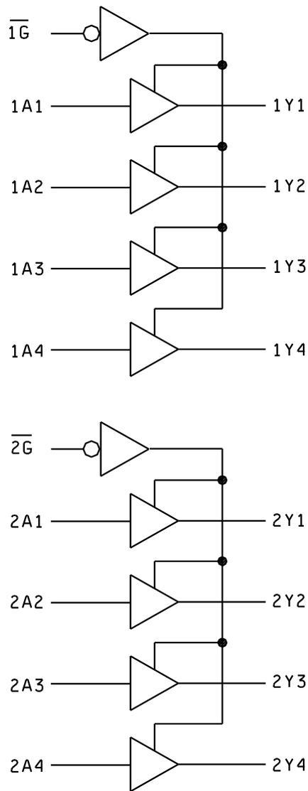
FIGURE 3. Logic diagram.
