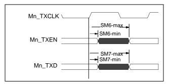
Figure 27 - GPSI Transmit Timing
