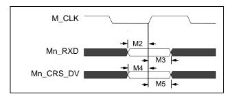
Figure 22 - RMII Receive Timing
