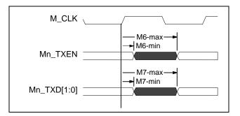
Figure 21 - RMII Transmit Timing
