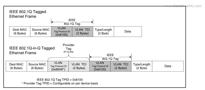
Figure 11 - Q-in-Q Tagged Ethernet Frame
