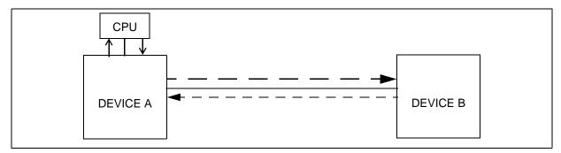
Figure 13 - Remote Loopback Test
