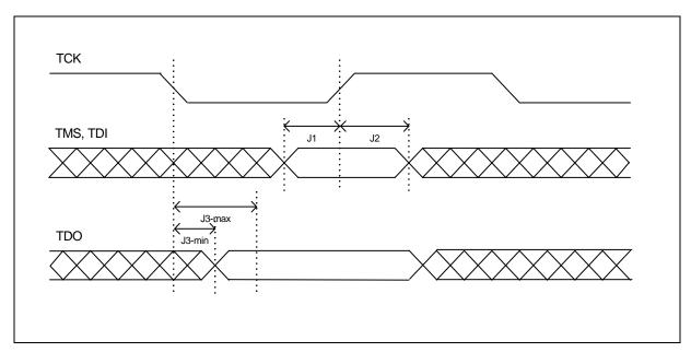
Figure 33 - JTAG Timing Diagram
