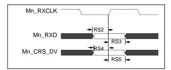
Figure 30 - RvGPSI Receive Timing
