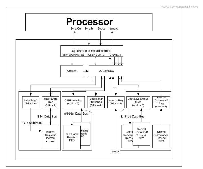
Figure 5 - Overview of the SSI Interface
