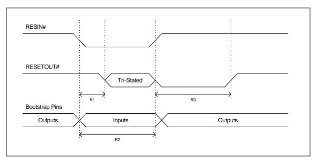
Figure 14 - Typical Reset & Bootstrap Timing Diagram
