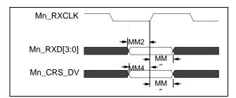
Figure 24 - MII Receive Timing
