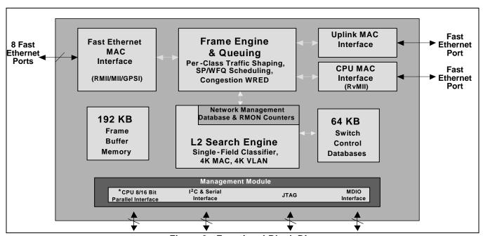
Figure 3 - Functional Block Diagram
