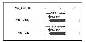
Figure 29 - RvGPSI Transmit Timing
