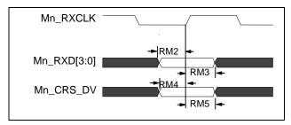
Figure 26 - RvMII Receive Timing
