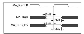
Figure 28 - GPSI Receive Timing
