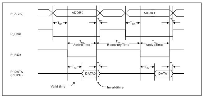
Figure 16 - Typical CPU Timing Diagram for a CPU Read Cycle
