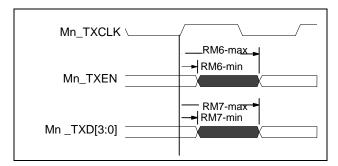
Figure 25 - RvMII Transmit Timing
