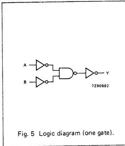
Fig. 5 Logic diagram (one gate).
