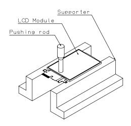
Fig. 8 COG Constant Pushing Test
