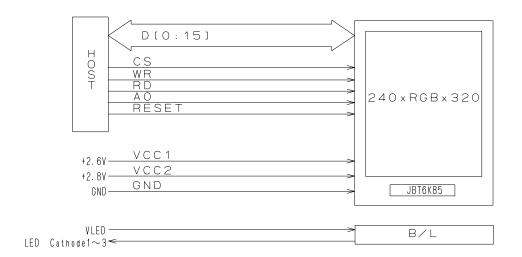
Fig.1 Schematic of LCD module system
