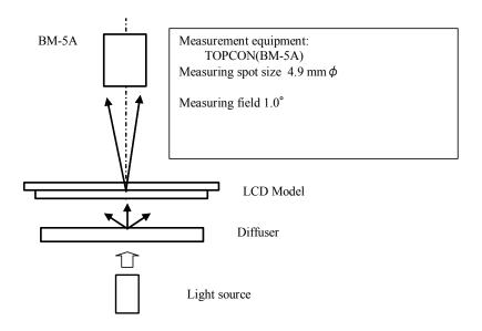
Fig. 3 Optical characteristics Test Method (Brightness)
