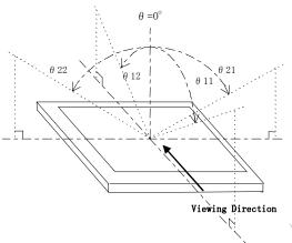
Fig .2 Definition of viewing angle
