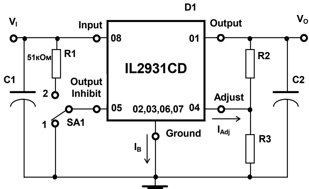
C1, C2 - input and output capacitance,
