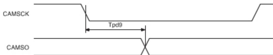
(within the recommended operating range, CAMSCK, CAMSO load capacitance = 29pF)
