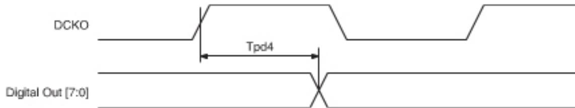
(within the recommended operating range, DCKO, PB[7:0] load capacitance = 15.5pF)
