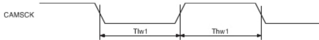
(within the recommended operating range, CAMSCK load capacitance = 29pF)
