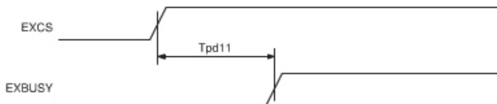
(within the recommended operating range, EXBUSY load capacitance = 20.5pF)
