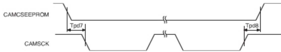
(within the recommended operating range, CAMSCK load capacitance = 29pF,
