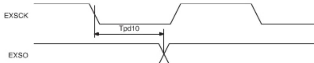
(within the recommended operating range, EXSO load capacitance = 20.5pF)
