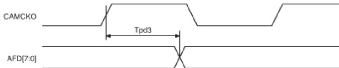
(within the recommended operating range, DCKO, PB[7:0] load capacitance = 14.5pF)
