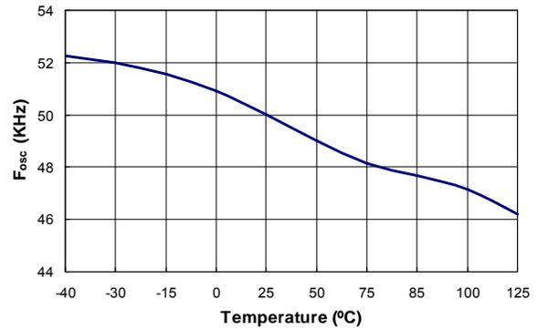
Figure 9. Center Frequency (f<sub>OSC</sub>) vs. Temperature
