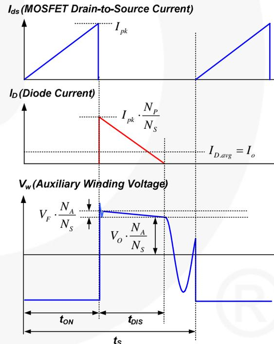
Figure 25. Key Waveforms of DCM Flyback Converter
