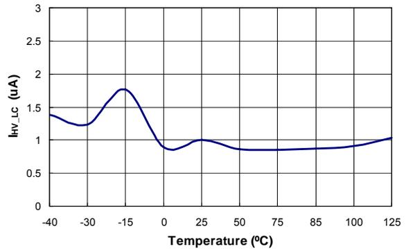
**Figure 21. Leakage Current after Startup (I<sub>HV-LC</sub>) vs. Temperature**
