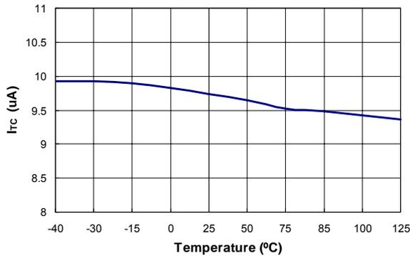
**Figure 18. IC Bias Current (I<sub>bc</sub>) vs. Temperature**
