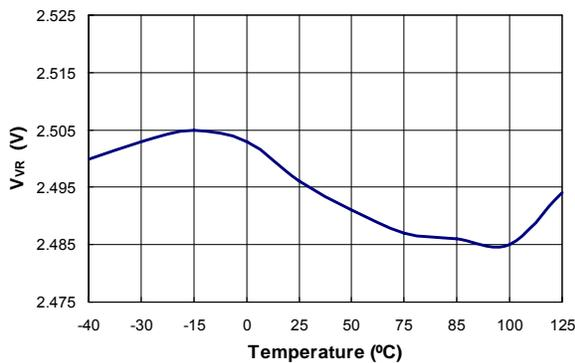
Figure 10. Reference Voltage (V<sub>VR</sub>) vs. Temperature
