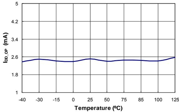
Figure 8. Operating Current (I<sub>DD-OP</sub>) vs. Temperature
