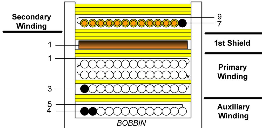
Figure 33. Transformer Specification
