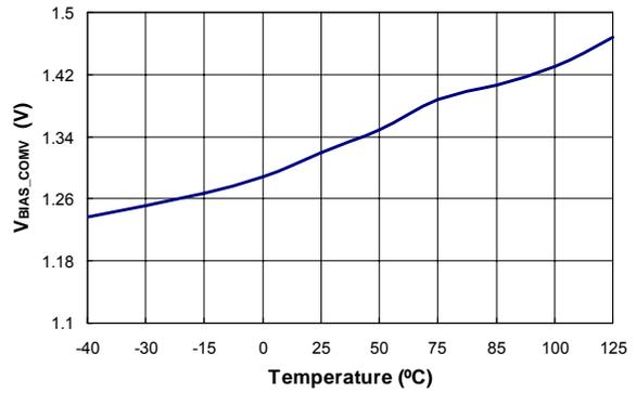
**Figure 19. Adaptive Bias Voltage Dominated by V<sub>COMV</sub> (V<sub>BIAS-COMV</sub>) vs. Temperature**
