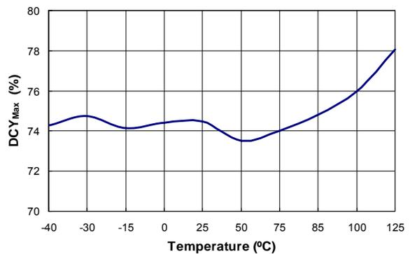
**Figure 23. Maximum Duty Cycle (DCY<sub>MAX</sub>) vs. Temperature**
