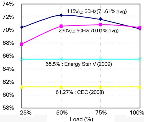
Figure 30. Measured Efficiency
